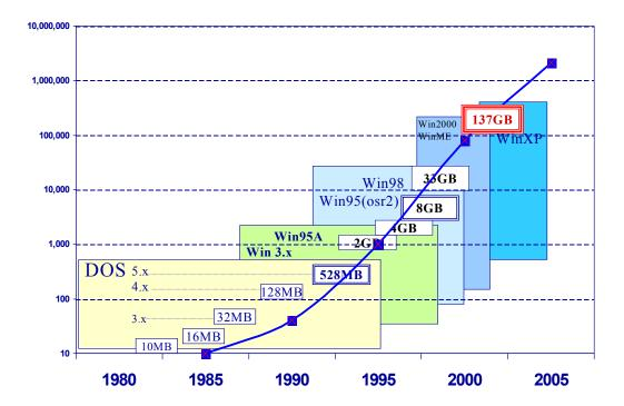
10 megabytes: early 16 megabytes: FAT 12 limit 32 megabytes: DOS 3.x limit 128 megabytes: DOS 4.x limit
