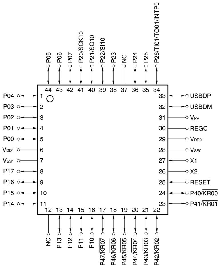
**Caution** In normal operation mode, connect the VPP pin directly to the VSS0 or VSS1 pin.
