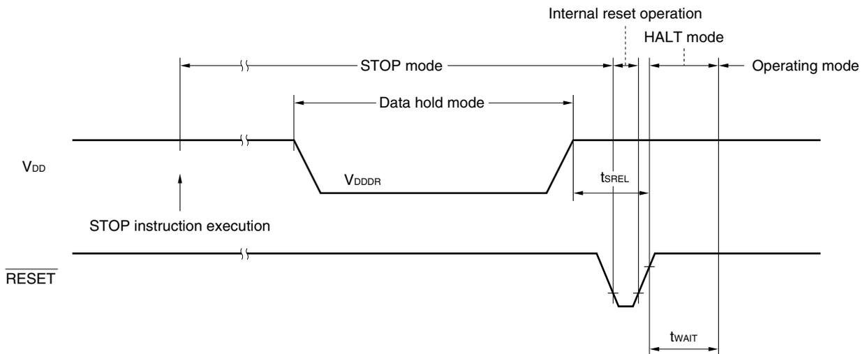
**DATA HOLD TIMING (standby release signal: STOP mode release by interrupt signal)**
