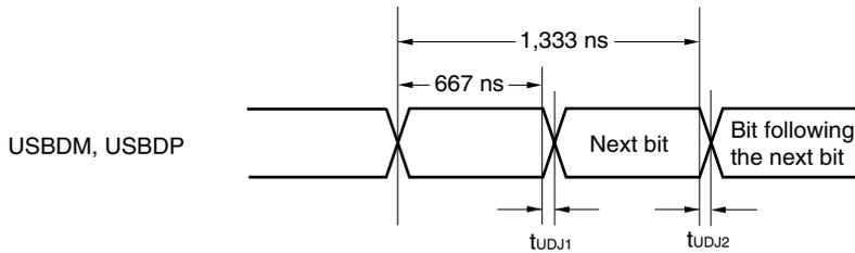
Differential output signal cross-over point, transmission EOP width, reception EOP width, and reception USB reset width
