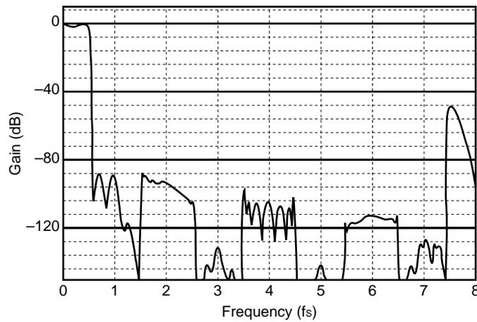
**Figure 3-7. Intraband Ripple Characteristics of Digital Filter**
