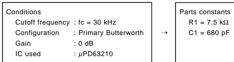
Figure 3-9. Configuration of D/A Converter Output Section (Configuration of Analog LPF)
