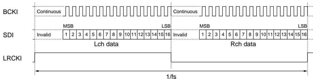
**Figure 3-4. Data Input Timing Chart (when BSEL = H)**
