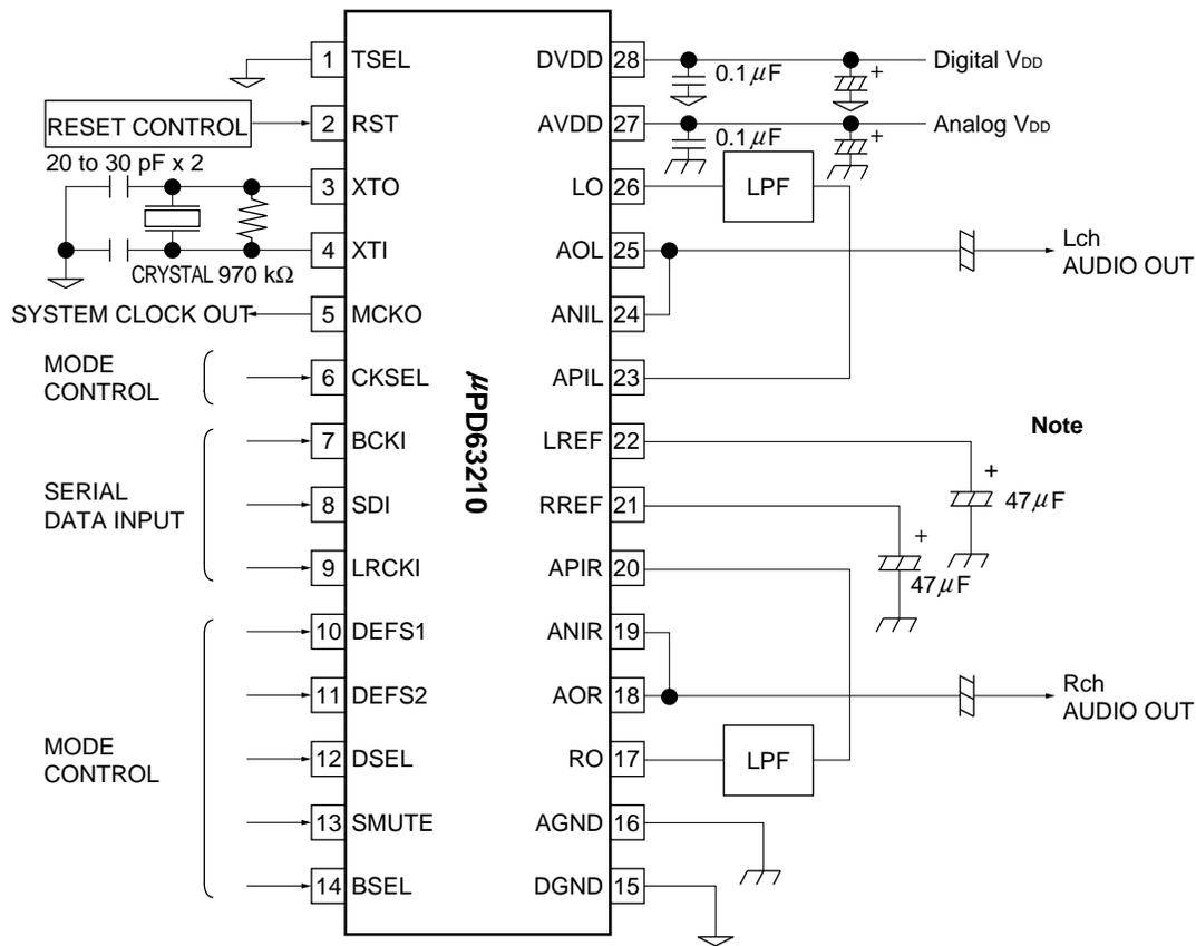
**Note** In this example, reference capacitors (21-/22-pin external capacitors) are installed independently. Even if these are realized in a common system (one 47μF), they will not cause any operational problems. However, the crosstalk may be deteriorated slightly (by several dB); therefore, please decide after evaluating the samples provided.
