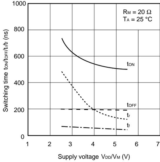
Switching time vs.  $T_A$  characteristics
