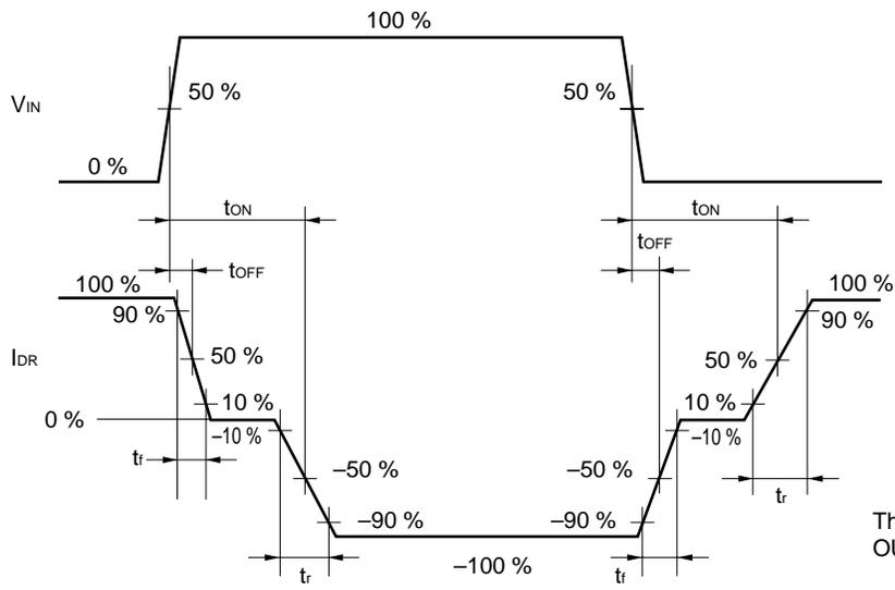
The current flowing in the direction from OUT\_A to OUT\_B is assumed to be (+).
