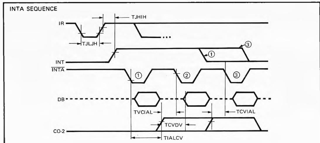
Notes: Interrupt output must remain HIGH at least until leading edge of first INTA.
