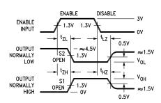
Diagram shown for Enable Low. Switches S1 and S2 open.
