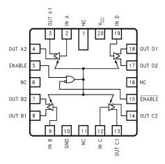
Figure 3. 20-Lead Ceramic Leadless Chip Carrier
