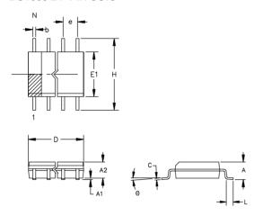
The chamfer on the body is optional. If it is not present, a terminal 1 identifier must be positioned so that 1/2 or more of its area is contained in the hatched zone.
