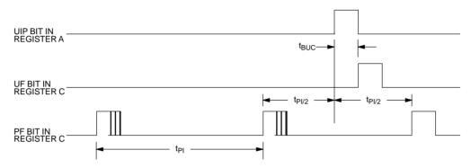
$t_{Pl}$  = PERIODIC INTERRUPT TIME INTERNAL PER TABLE 1  $t_{BliC}$  = DELAY TIME BEFORE UPDATE CYCLE = 244  $\mu$ s
