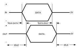
Figure 4. Transmit IDLE-DATA and DATA-IDLE Response Time
