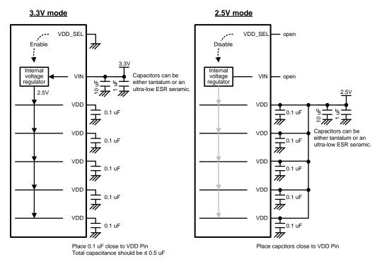
Figure 6. 3.3V or 2.5V Supply Connection Diagram
