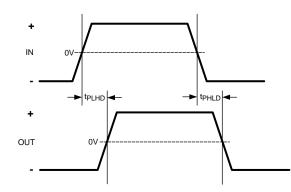
Figure 3. Propagation Delay Timing Diagram
