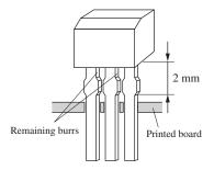
When soldering the leads, remember to separate the soldering position by 2 mm or more from the resin part of the package.
