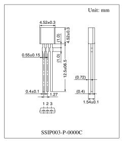
Note) The package of this product will be changed to lead-free type (SSIP003-P-0000J). See the new package dimensions section later of this datasheet.
