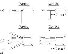
Bending position of lead wire
