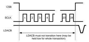
The DAC Configuration command LDAC (see Section 1.12 INSTRUCTION SET below) will also update the DAC output as soon as it is received. The effect of hardware LDACB or software LDAC is the same i.e. data is transferred from the PREREG to DACREG and output of the DAC is updated.
