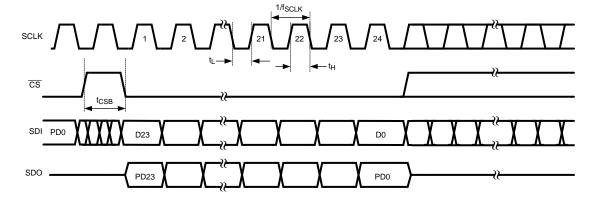
Figure 1. DAC161S055 Input/Output Waveforms
