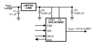
Figure 4. Using the LM4120 as a power supply
