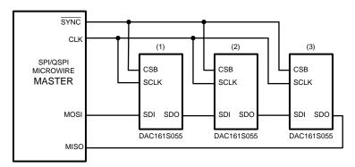
A sample of SPI data transfer appropriate for a 3 DAC Daisy Chain is shown in the figure below.
