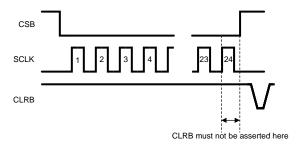
Clear function can also be accessed via the software instruction CLR, see Section 1.12 INSTRUCTION SET below. The effect of hardware CLRB or software CLR is the same.
